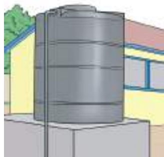
Polytank used to store water
