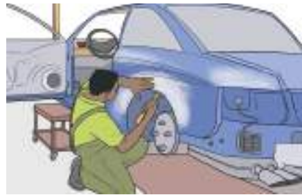
A welder hitting a dented car body to straighten it
