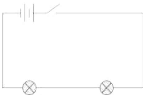
Fig. 6 - Two bulbs in series with a battery of two cells
